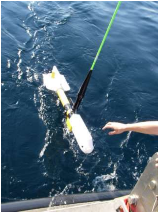
Magnetometer being towed by a ship
